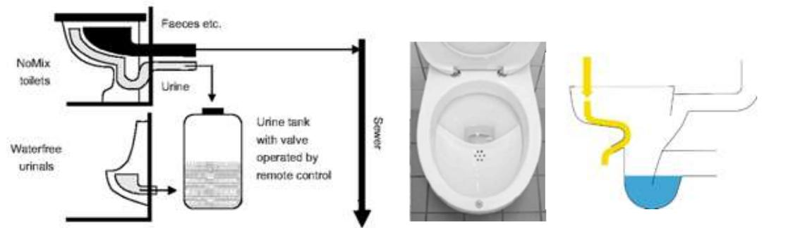
Figure 1. Principles of urine source separation technology and example of two toilets with and without (type Laufen: SAVE) a separate bowl for urine collection.
