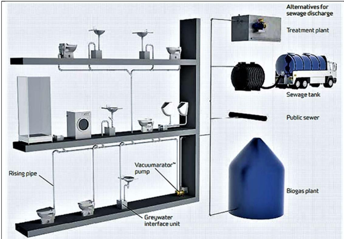
Figure 1. System design example with various discharge options. (Source: JETSGROUP, 2013)
