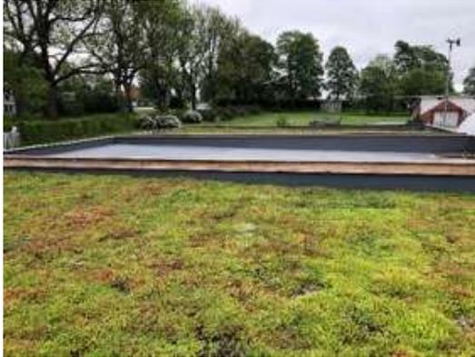
Figure 1. Green roof real scale test laboratory with sedum spp and 15 cm lightweight aggregates at NMBU, Campus Ås, Norway.
