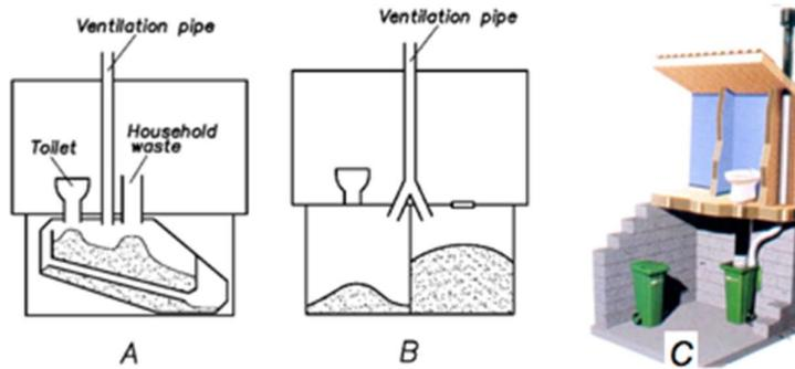
**Figure 1.** Dry/composting toilets. A: single chamber, B: dual chamber, C: removable chambers
