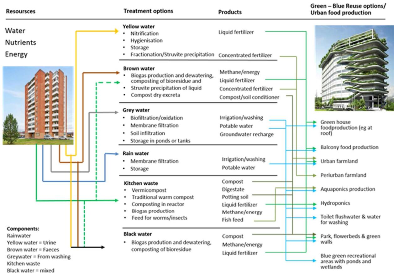
Fig. 1. SiEUGreen model of recyclable resources
