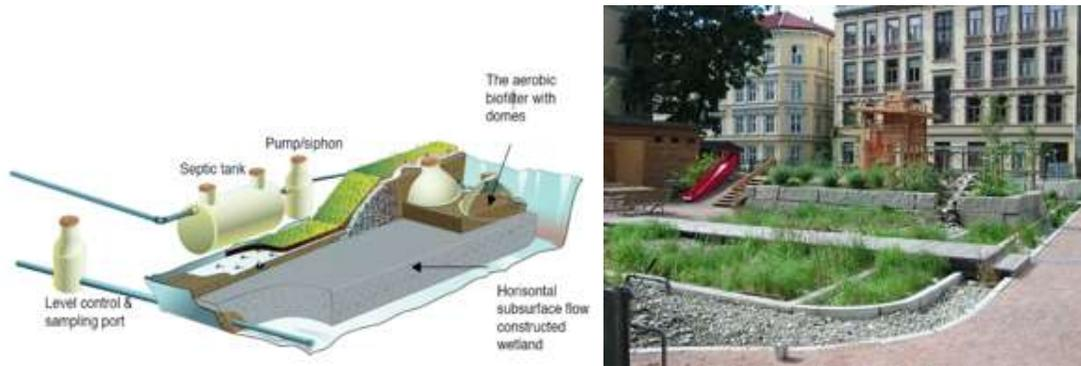
Figure 1. Filterbed system with integrated aerobic biofilter for greywater treatment (Jenssen and Vråle, 2003) and a biofilter combined with constructed wetlands for greywater treatment in Oslo
