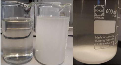
Figure 1. Struvite precipitation from anaerobically treated source-separated blackwater at the NMBU laboratory.
