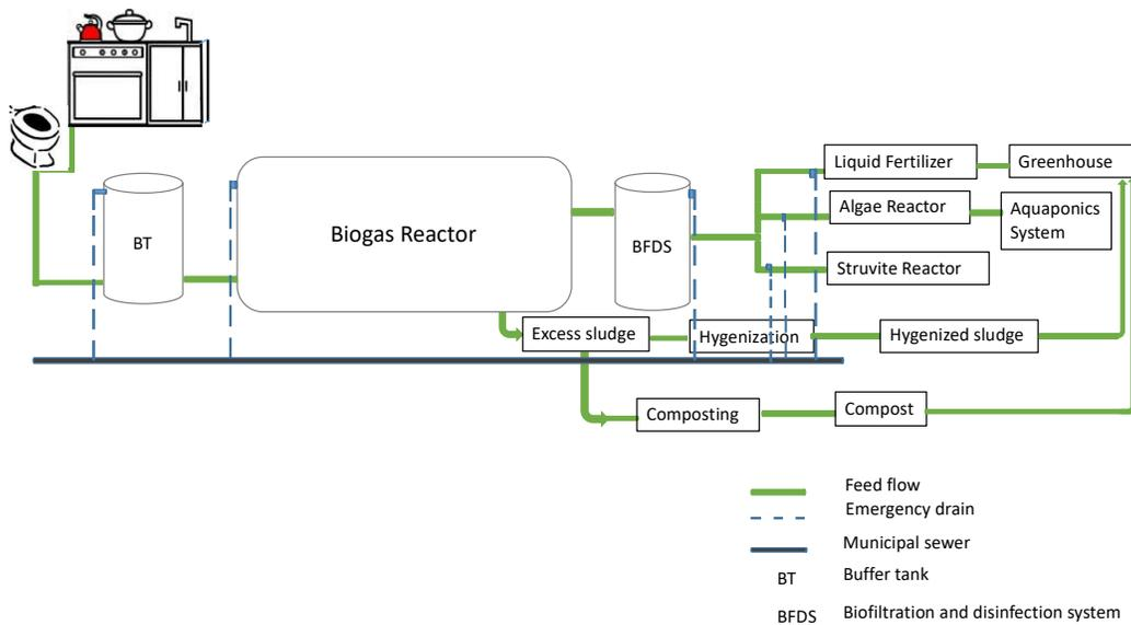
Fig. 3. Schematic plan of the treatment system for organic household waste and blackwater in Fredrikstad.
