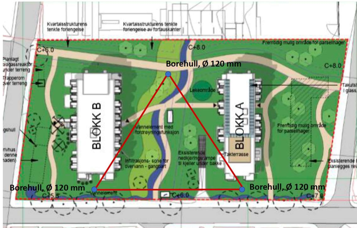
Fig. 7. Location of the wells drilled for investigating borehole thermal energy storage (BTES).
