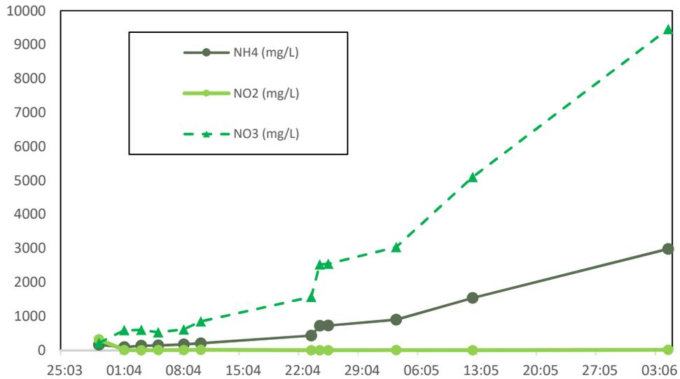
Figure 4. Ammonium, nitrite and nitrate in the biofilter product. Input was diluted urine: increasing gradually from 5% to 50% substrate in the period 28.03 to 05.06.
