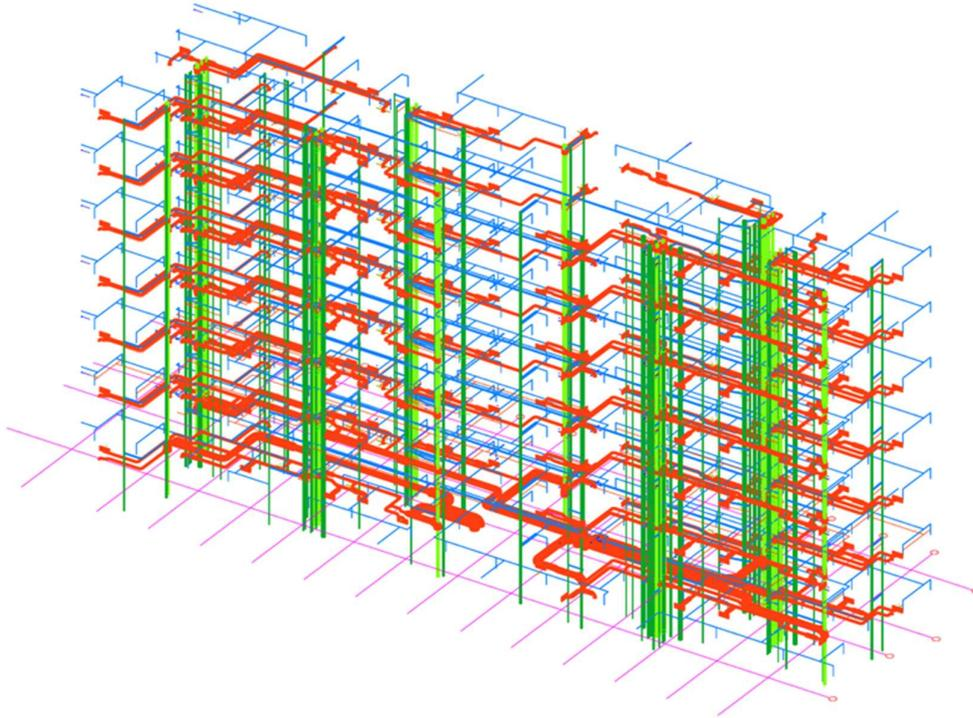
Fig. 2. Plan for pipes in the Fredrikstad showcase.
