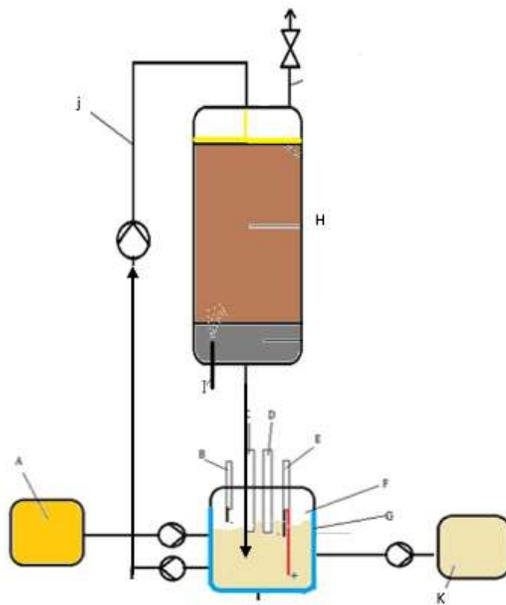
Figure 2: Biofilter laboratory trial: A = substrate, C-E = sensors, O<sub>2</sub>, pH, F = intermediate tank for sensor and mixing, G=cooling liquid for temperature control, H=Biofilter with porous media, I = air inflow and outflow on top of reactor, J= tube with pump to make the solution circulate, K= product storage tank (pumps were controlled by pH set point in A and K). Control system was similar to bioreactor.
