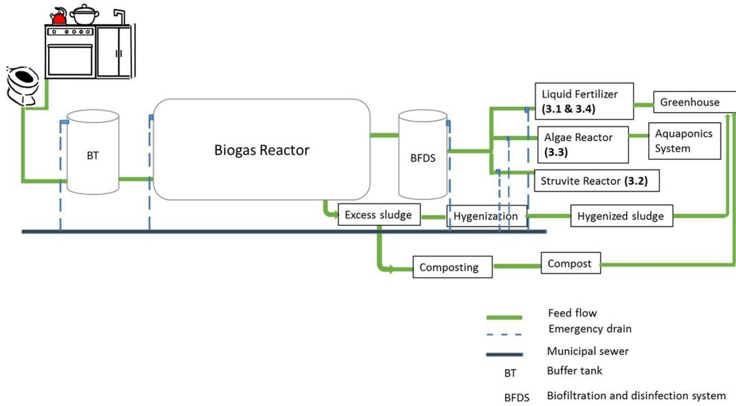
Fig. 2. Schematic plan of the treatment system for organic household waste and blackwater in Fredrikstad.
