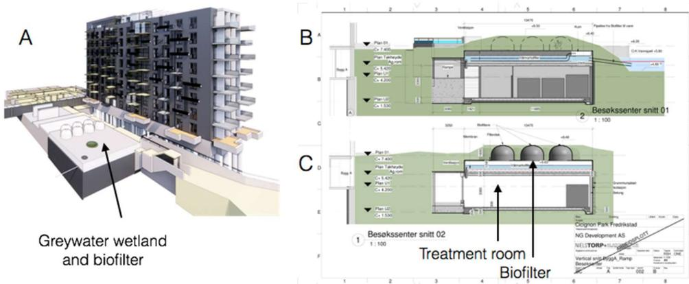
Fig. 6. The greywater wetland and biofilter. A: 3D drawing, B: Cross section west-east, C: Cross section south-north.
