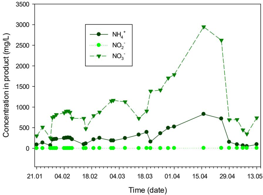
Figure 3: Ammonium, nitrite and nitrate in product in moving bed bioreactor. Input was to start with diluted urine: 21.-28.1: 5%, 29.1-8.2: 10%, 9.-19.2: 20%, 21.2-7.3: 10%, 8.3-1.4: 15%, 2.4-24.4: 25%. Then input was changed to digestate: 25.4-13.5: 25%.
