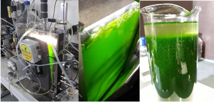
**Figure.** Bench scale flat panel PBR for continuous *C. sorokiniana* cultivation using treated and diluted anaerobically treated blackwater (Photo: Melesse E.)
