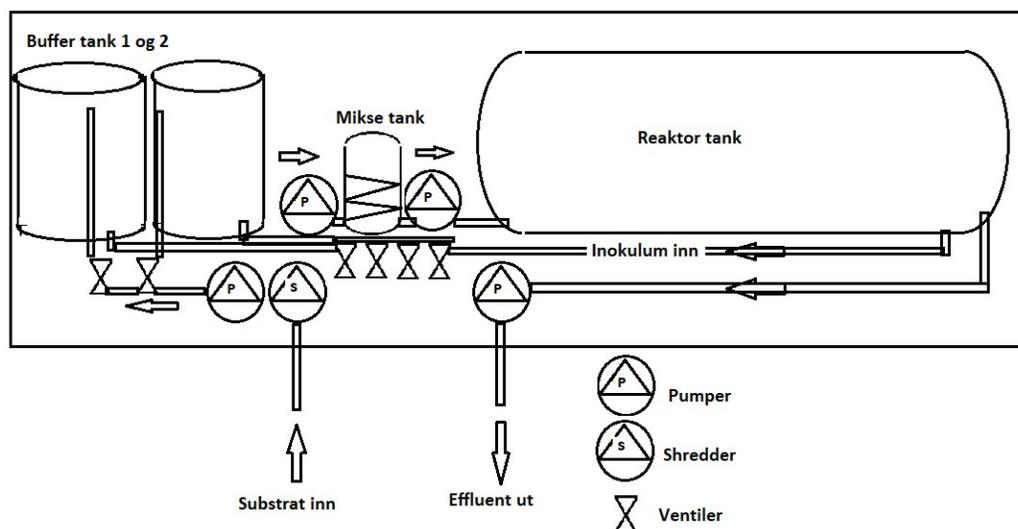
Figure 7. Biogas production reactor.
