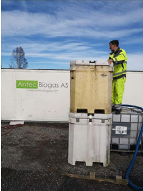
Figure 9. How containers were arranged for dewatering of digestate.
