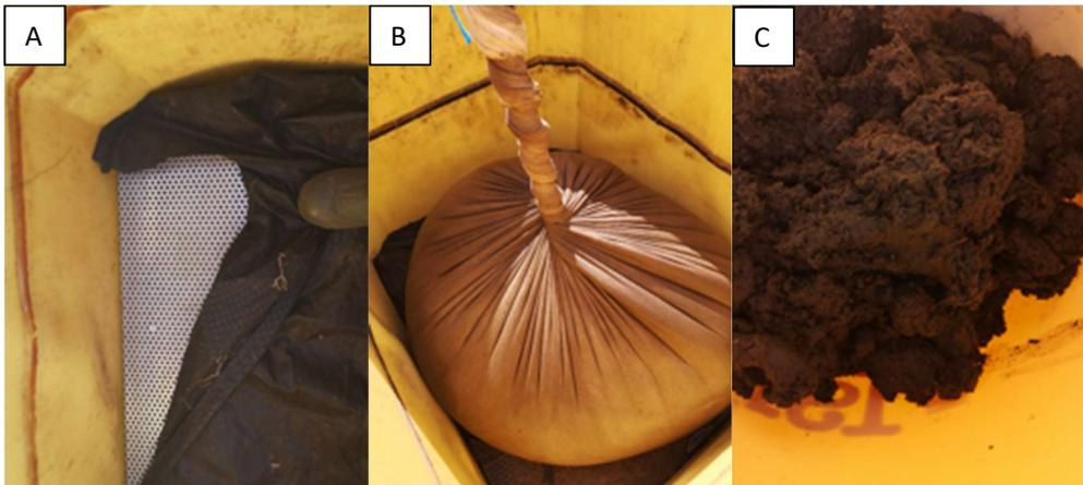
Figure 10. Illustration of the dewatering process and the final digestate ready for composting. The liquid part was collected and used for biofiltration experiments (e.g. nitrification).
