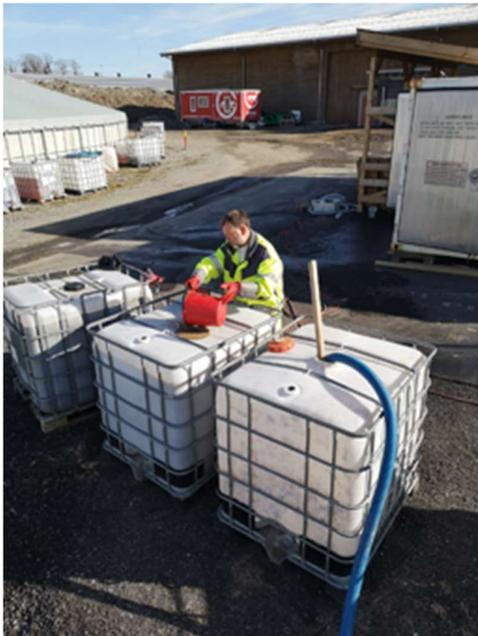
Figure 8. The addition of HFW to PS. The blue tube was used for pumping feedstock mix into the buffer tanks inside the container.
