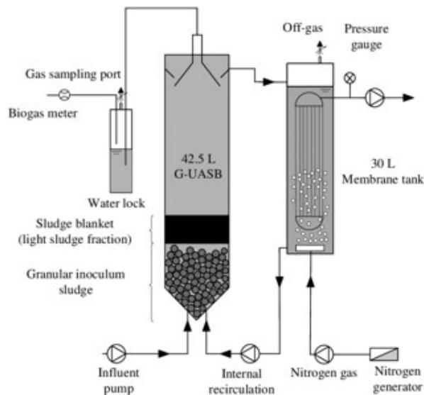
Figure 2. Anaerobic membrane bioreactors.
